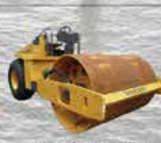
Vibratory Roller Valvo SD100D (10 Ton)
