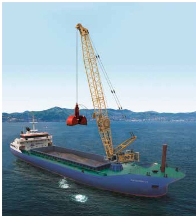
Above: The HS 8300 HD is the largest duty cycle crawler crane in Liebherr's HS series.
