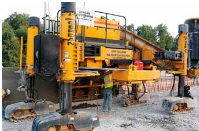
A 2,268 kg counterweight package was positioned on the right side of the paver.
