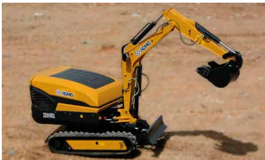
The new XCMG XE15R hydraulic 'intelligent' excavator is a fully remote-controlled machine.
