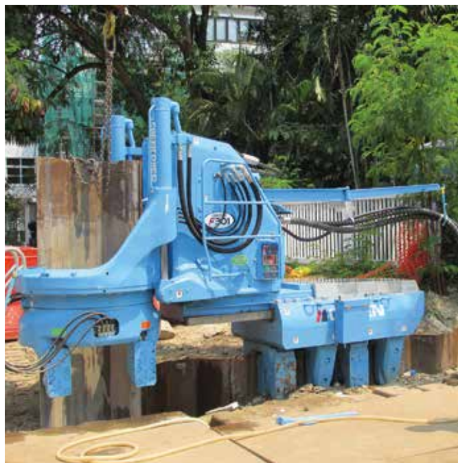
Top, above and left: Giken's F301 silent piler with hat type sheet pile 900 being used on a drainage project in Singapore. This versatile machine can be modified to suit various soil conditions and working environments.
