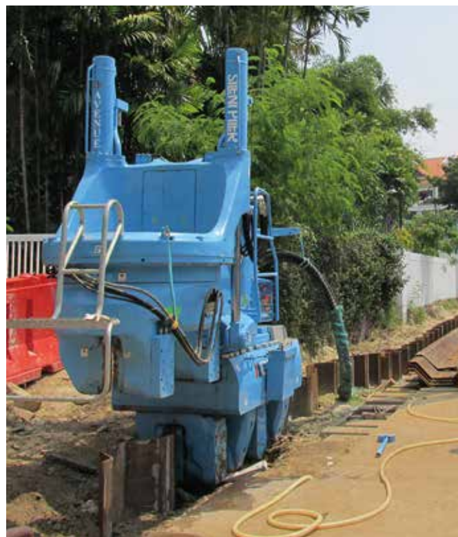
Top, above and left: Giken's F301 silent piler with hat type sheet pile 900 being used on a drainage project in Singapore. This versatile machine can be modified to suit various soil conditions and working environments.
