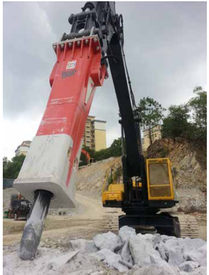
Above: Crescendo Infra is using a Rammer 5011, mounted on a 45 t class Volvo E460 excavator, to break exceptionally hard granite on a residential project in Malaysia.
