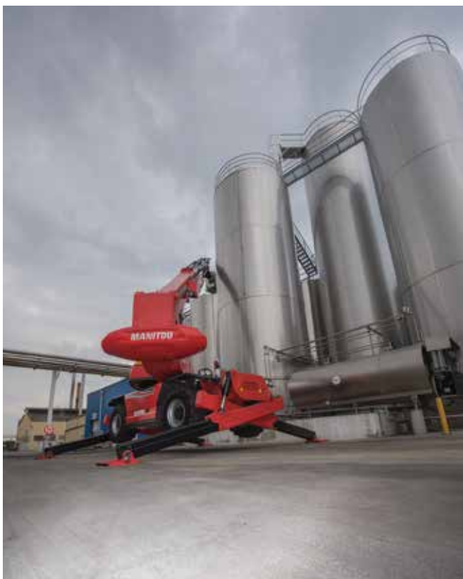
ABOVE AND LEFT: Well suited to heavy high-rise construction, the MRT 2470 rotating telehandler has a lifting capacity of 7 t and a maximum reach of 24 m. The machine won an Intermat Innovation Award earlier this year for its stabilisation system.
