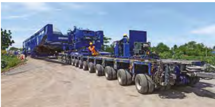
Silamas on the road with Goldhofer 2x16 THP/SL axle lines and Faktor 5 high girder bridge.
