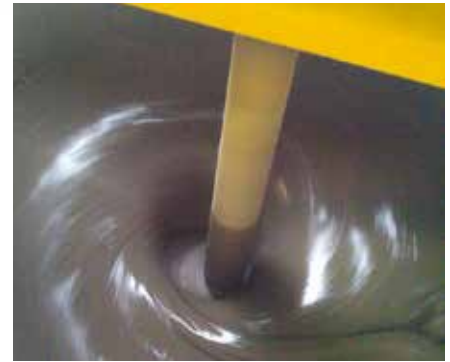
The CG-460 has variable-speed, high-shear disks that rotate up to 3,000 rpm for excellent mix consistency.
