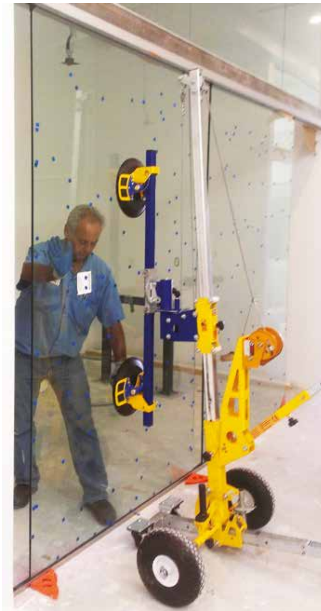
LEFT: Quattrolifts' new Express 150T allows users to lift glass weighing up to 100 kg above doorways and entrances with greater safety and efficiency. The machine can be easily transported to site by one person.
