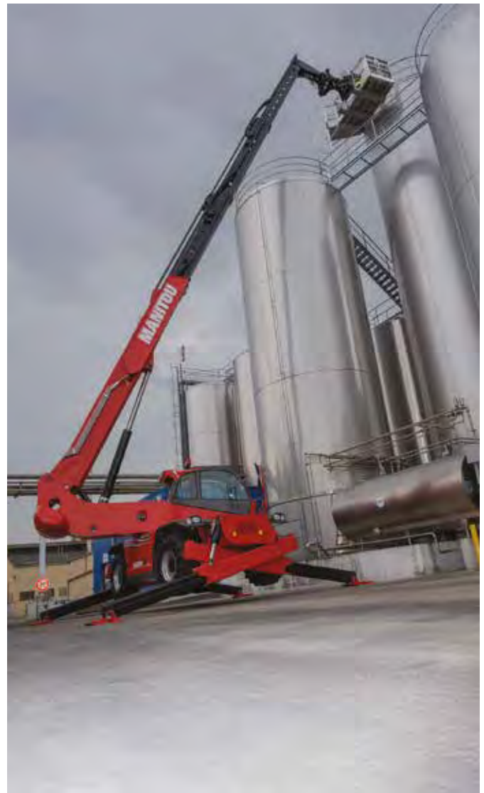
ABOVE AND LEFT: Well suited to heavy high-rise construction, the MRT 2470 rotating telehandler has a lifting capacity of 7 t and a maximum reach of 24 m. The machine won an Intermat Innovation Award earlier this year for its stabilisation system.
