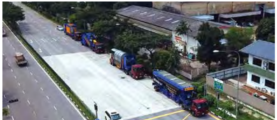
ABOVE: The basic Linnhoff mobile asphalt plant unit consist of four modules with built-in axles. These four modules can be seen here being transported on their prime movers.
