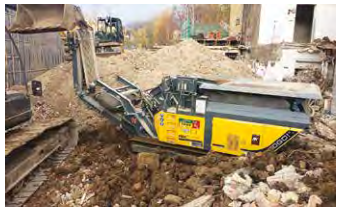
ABOVE AND LEFT: The RM 70GO! 2.0 crushes 125 t/hr quietly with low emissions near the Camden Market in London. The machine can easily drive through narrow gateways and restricted areas.
