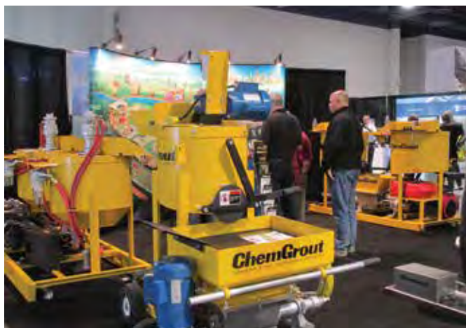
ChemGrout manufactures a wide range of standard and custom-built grouting equipment to handle various materials and capacities (from 3.8 to 284 l/min), with pressures from 3.4 to 138 bar.
