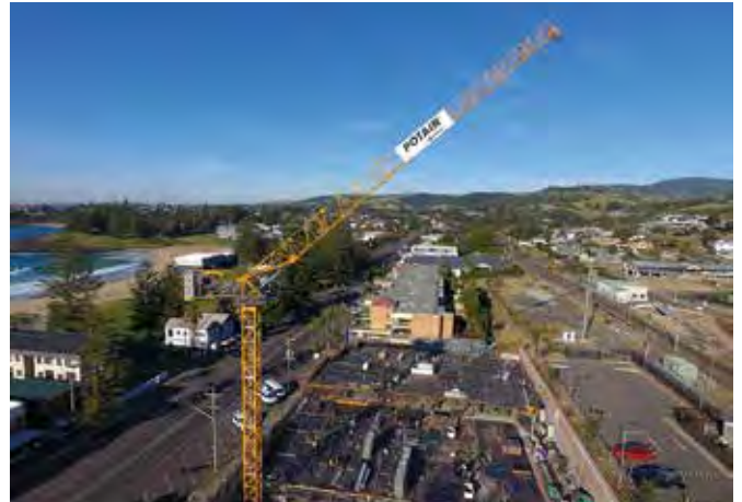
Manitowoc's new topless luffing jib crane, the Potain MCH 125, is believed to be the first in the world to use hydraulic power for its articulating movement.
