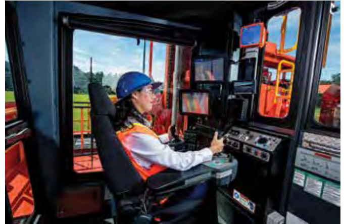
ABOVE: Sandvik DR412i blasthole drill is automation-ready and is designed for rotary and down-the-hole drilling applications with a hole range of 216-311 mm. The picture here shows the DR412i cabin.
