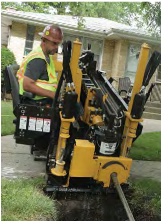
Vermeer's new D8x12 Navigator horizontal directional drill features a low noise emission level of 85 dBA and sound power of 104 dBA, making it excellent for use in urban areas.
