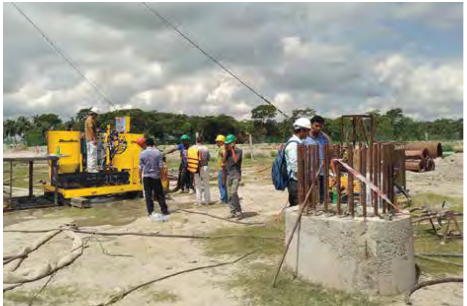
TOP: ChemGrout's CG-680 high-pressure, high-capacity, skid-mounted colloidal grout machine is designed for mixing and pumping slurries of cement, fly ash, bentonite and lime flour.
